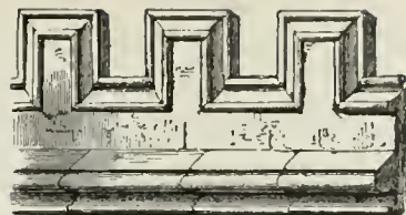
PARAPET CUT INTO SMALL CRENELLATIONS IMITATING BATTLEMENTS; S. PETER'S CHURCH, DORCHESTER, ENGLAND; c. 1450.
